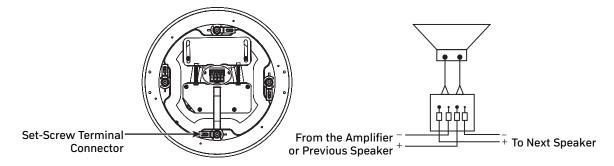
3. Strip the insulation on each conductor back 1/4" and use the small flathead screwdriver to secure each wire into the connector.
