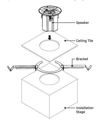
the mounting dogs clamp onto the ring. Be careful, overtightening the screw can damage the ceiling tile and/or the speaker.
