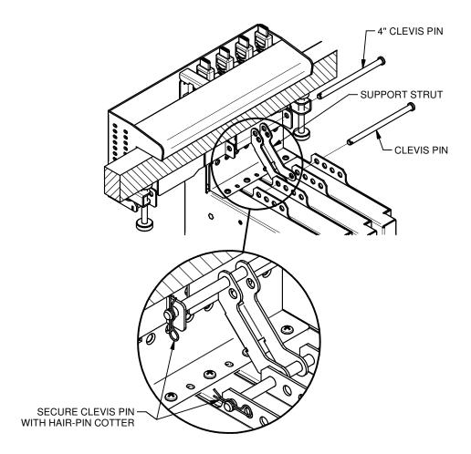
R-3. FOR ADDITIONAL TAMPER-PROOF INSTALLATION, INSTALL #6-32 x 1/4 LONG PAN HEAD SCREW. REINSTALL RT6-CL2 ASSEMBLY TO TABLE.
