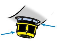
The locking nut tightens the seal around the cabling. The thin nut secures the connector to the extension mount.
