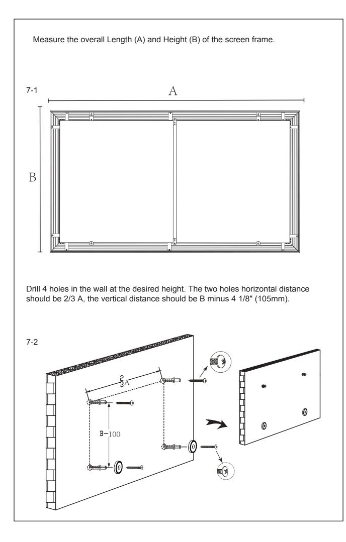
Hammer the expansion bolts into the 4 drilled holes, and drive 2 round head self-tapping screws into the upper expansion bolts, leaving about 1/4" (5mm) extended for hanging the screen on. Install the lower 2 magnet pieces using 2 flat self-tapping screws. Hang the screen on the upper brackets and attach the lower frame to the wall using the magnets.
