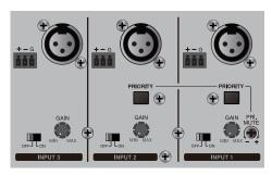
(1) PHANTOM Switch: If you want to use a condenser microphone, turn this switch on to provide DC 24V PHANTOM power.
