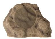
OSR85 Part: OSR8500 Woofer: 8" Injection Polypropylene with Rubber Surround Tweeter: 1" Titanium Power RMS: 50 Watts Power Peak: 100 Watts Frequency Response: 40Hz – 20kHz Impedance: 8 ohm, 70v – 60W/30W/15W/7.5W transformer taps Dimensions: 15 x 21 x 16" (38 x 52 x 39 cm) Weight: 11 lbs (5 kg) Environment Temp: -22° to 158° F (-30° to 70° C)
