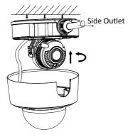
Figure 2-3 Route the Cables via Side Outlet
