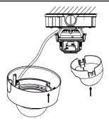
Figure 2-4 Install the Black Liner and Bubble
