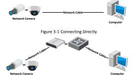
Figure 3-2 Connecting via a Switch or a Router
