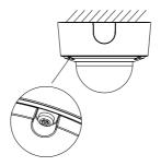
Figure 2-5 Tighten the Lock Screw
