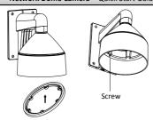
Figure 2-7 Install the Rubber Ring and Screws
