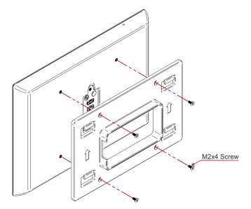
Figure 12: Attaching the Panel Mount Plate to the Rear Side of the KT-107S
