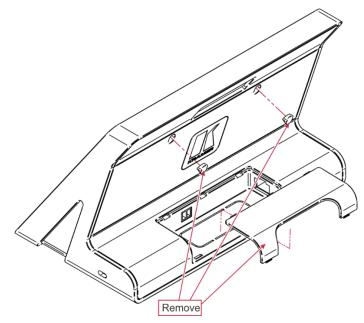
Figure 6: Removing Cable Cover and Rubber Screw Cover
