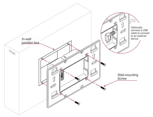
Figure 10: Installing the On-Wall Mount Unit
