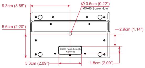
Figure 5: Cut-Out Dimensions (image not to scale)
