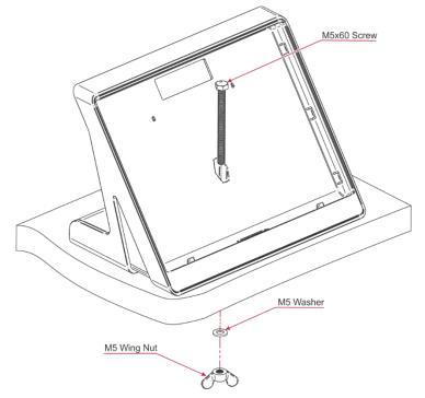
Figure 7: Securing Tabletop Mount
