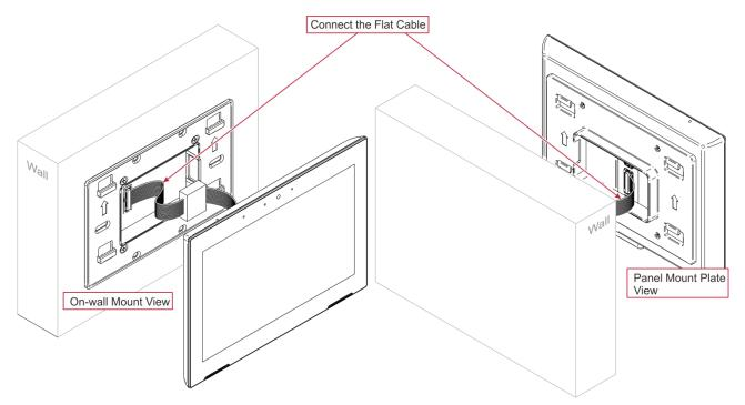
Figure 13: Connecting the On-wall Mount Flat Cable
