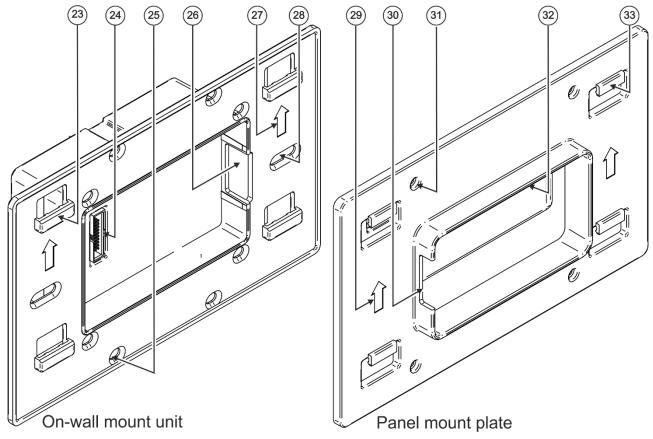
Figure 4: KT-107S Touch Panel Front Panel
