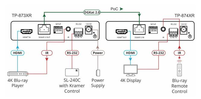
Figure 3: Connecting to the TP-873XR/TP-874XR Rear Panel
