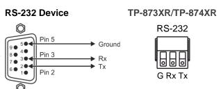
9-pin D-sub Female Connector (from PC)
