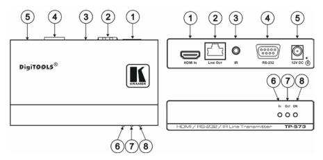
Figure 1: TP-573 HDMI/RS-232/IR Line Transmitter
