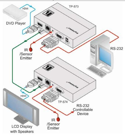
Figure 3: Connecting the TP-573/TP-574 Transmitter/Receiver
