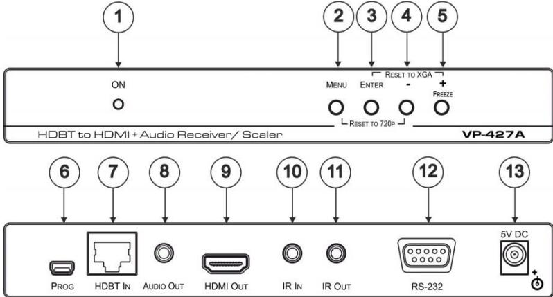
Figure 1: VP-427A HDBaseT to HDMI+Audio Receiver/Scaler
