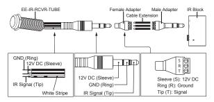
When using long lengths of cable (>50ft.), it may be necessary to connect a 470 0hm 1/8 Watt resistor between the "IR IN" (signal) and "GND". The resistor discharges the cable capacitance, which allows high bit-rate IR codes to work with higher reliability.
