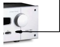
4. Self-adhesive "Flashers" affix to the Infrared sensors on the front panels of your components. The Flashers relay commands to components out-of-sight of the MRF-350's Front Blaster. The flashers plug in to the MRF-350's rear flasher line outputs via their 10 foot cables. Uniquely, the MRF-350 can also connect to components with rear panel IR Inputs via its adjustable IR Line Outputs.
