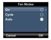
If the **Fan Modes** screen times out and goes back to the main screen without pressing the **OK** button, no change is made to the fan mode
