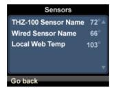
The second list entry is any wired sensor in the system. The name of the sensor is displayed with the current reading to the right. If there is no wired sensor in your system then this line is not displayed.
