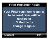
Press the key below the **OK** key label in the smart-key label at the bottom right of the display to reset the reminder. If you decide to cancel the operation then press the key below the **Cancel** key label in the smart-key label at the bottom left of the display.
