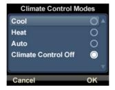
In **Cool** mode, the thermostat activates the system equipment to cool your home per the programmed schedule or hold temperature. The thermostat does not activate the system equipment to heat your home while in the **Cool** mode.
