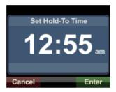
When you have selected the desired time press the key below the **Enter** key label in the smart-key label at the bottom right of the display to select this new mode. If you decide to cancel the operation then press the key below the **Cancel** key label in the smart-key label at the bottom left of the display.
