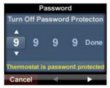
At the bottom of the screen are three smart-key labels for the three buttons located below the LCD display. The left button is **Cancel**, the center button is a left arrow, and the right button is a right arrow.
