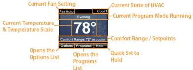
The center of the screen displays the current temperature with different backgrounds dependant upon whether the thermostat is in Heating, Cooling or Idle mode. The small letter **F** or **C** at the lower right of the current temperature indicates the temperature scale.
