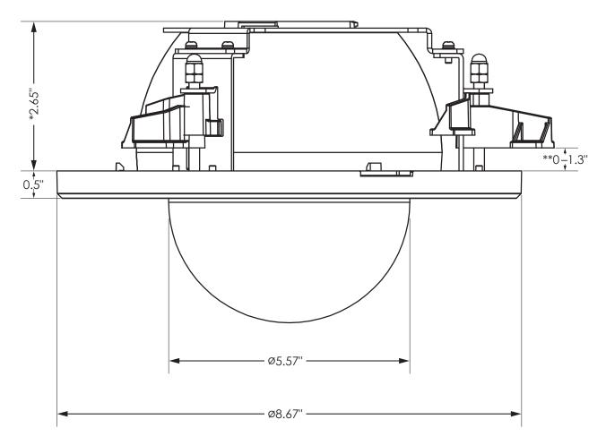
\* Dimension includes height of camera installed in the bracket.
